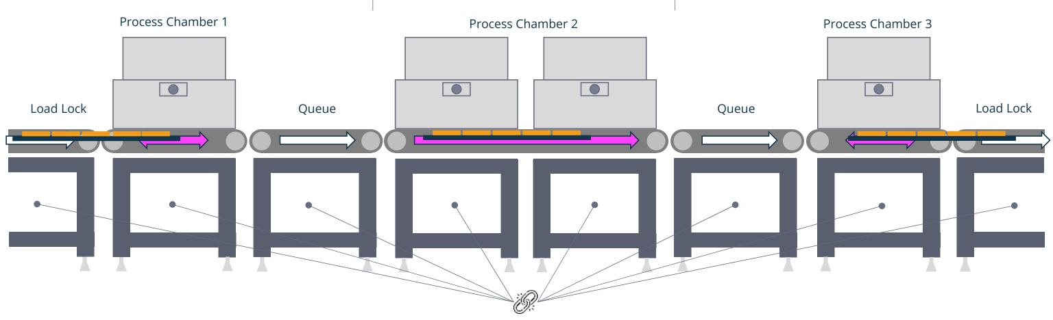
All common modules linked to form a linear system One vacuum chamber for whole transportation system
